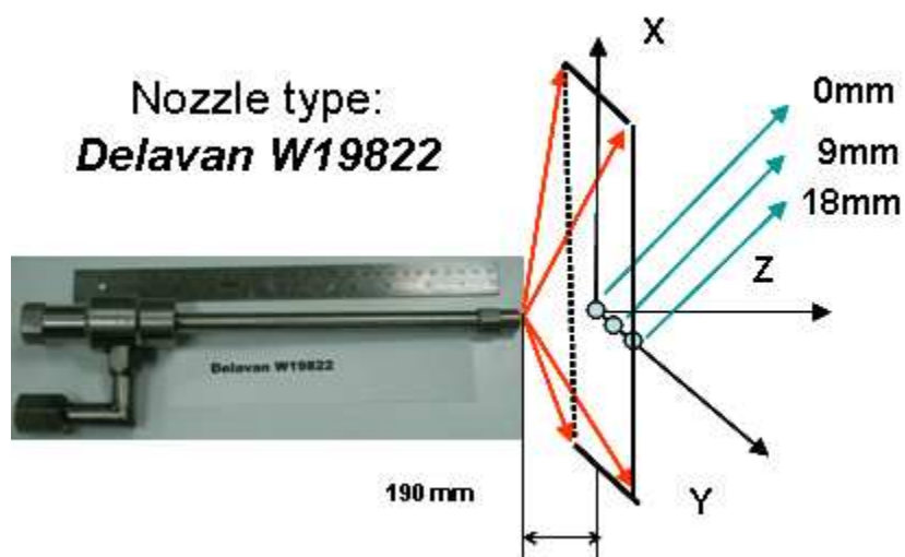
Fig. 3.6 Delavan Nozzle W19822 and Three Sample Locations ( Y=0, 9, 18\text{mm} ) Investigated During Experiments
