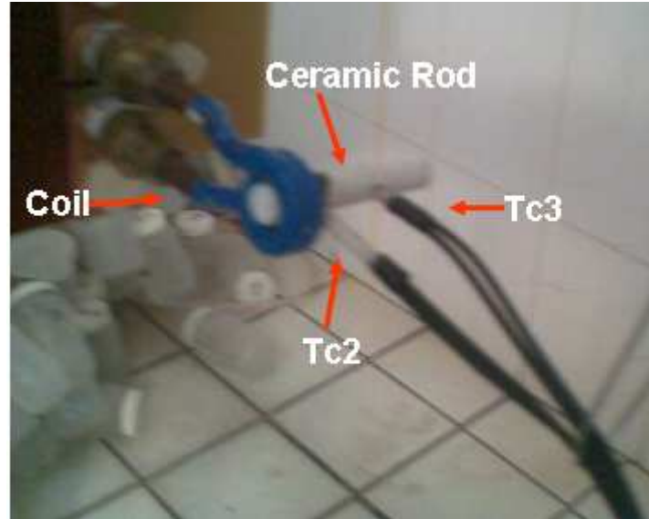
Fig. 5.19 Experiment Setup for Investigation Magnetic Field Effect on Thermocouples Measurements
